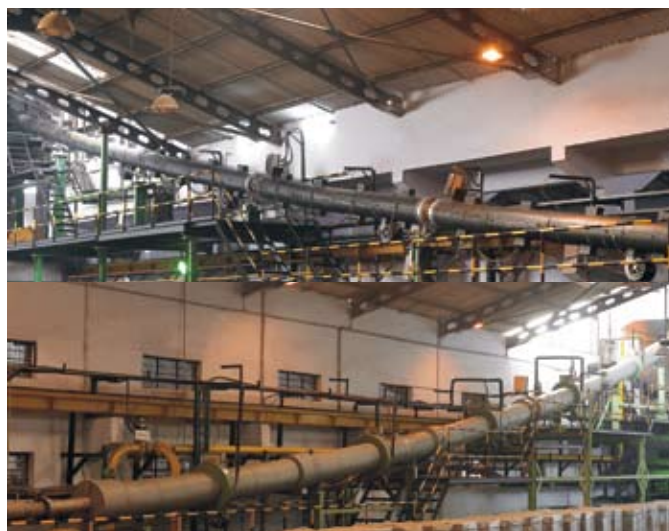
Figure 1 : 2 CCV (DRY CURE) LINES
