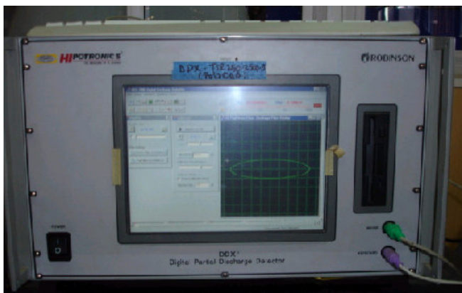
COMPUTERISED PARTIAL DISCHARGE DETECTOR
