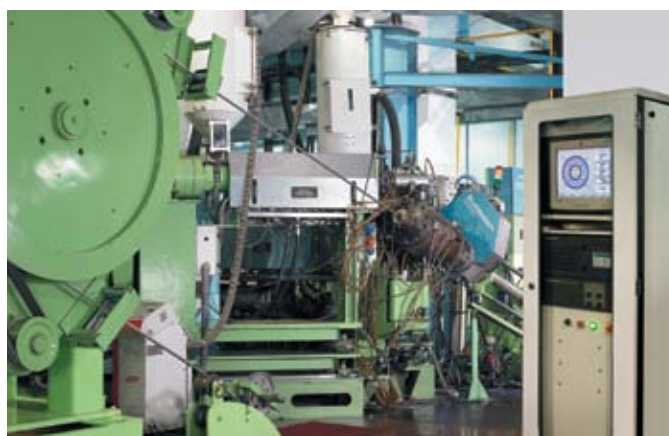
Figure 2 : THREE LAYER COMMON TRIPLE EXTRUSION METHOD
