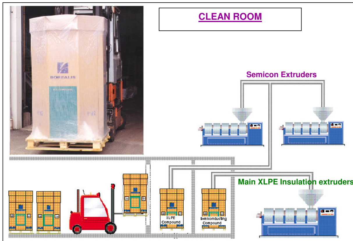
XLPE CONTAINER TRANSPORTATION TO MANUFACTURING LINES
